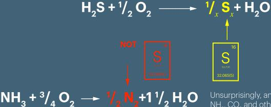
Unsurprisingly, an SRU **does not** convert NH<sub>3</sub>, CO<sub>2</sub> and other non sulfur species into **sulfur**. If NH<sub>3</sub> is not destroyed in the SRU Reaction Furnace (as it is in all Bechtel-licensed Sulfur Plants), then it will precipitate, forming
