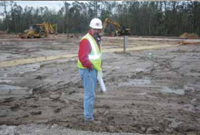
Photo 1 | Robert Jordan is shown here evaluating the soil strength on a soft, wet site using the “sink” criteria.
